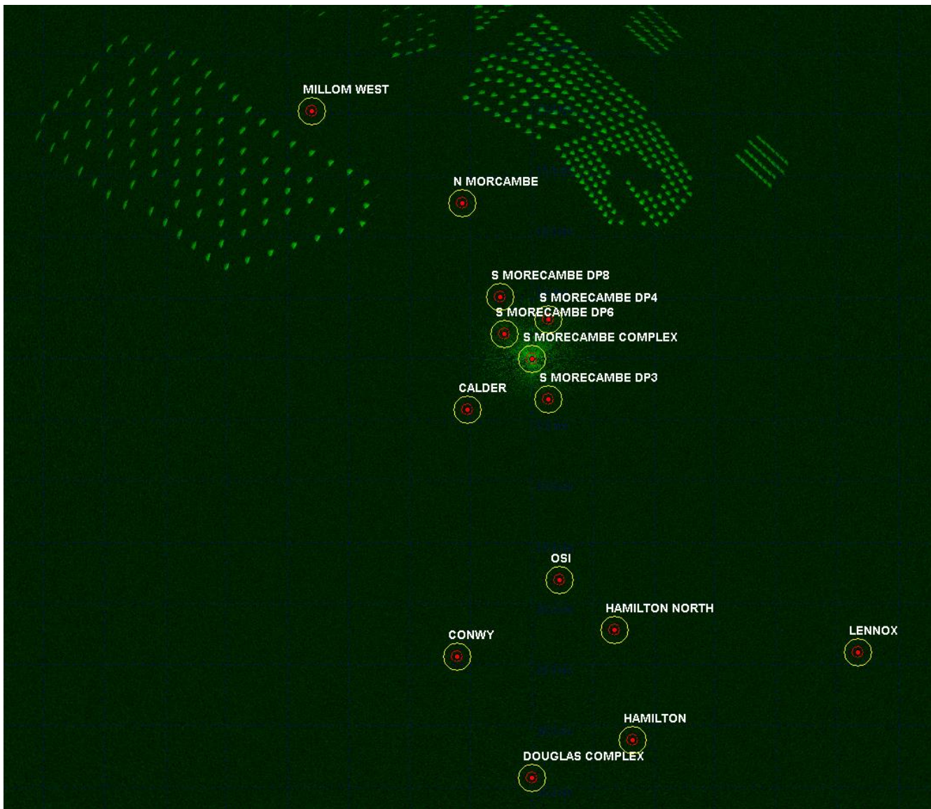
Figure 1.36: Spirit Energy’s South Morecambe AP1 platform REWS clutter map showing returns from the Morgan wind turbines and sea clutter.
