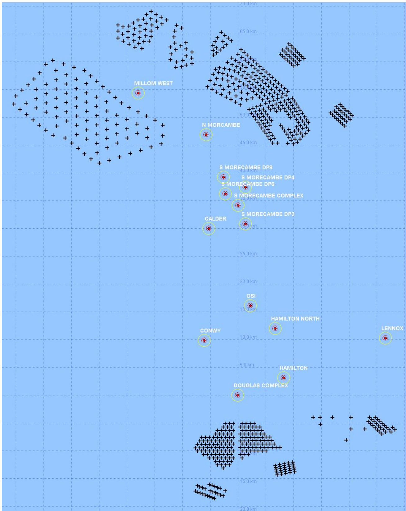
Figure 1.26: Modelled layout of the Morgan Generation Assets showing the indicative location of the wind turbines and the location of oil and gas platforms in the region.
