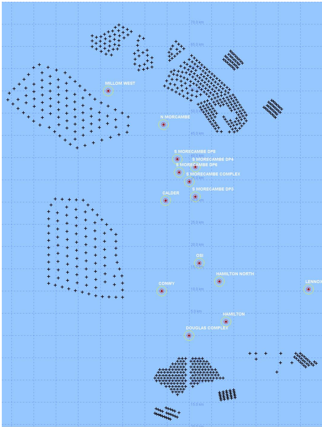
Figure 1.40: Modelled cumulative layout of the Morgan Generation Assets and Mona Offshore Wind Project showing the indicative location of the wind turbines and the location of oil and gas platforms in the REWS study area.
